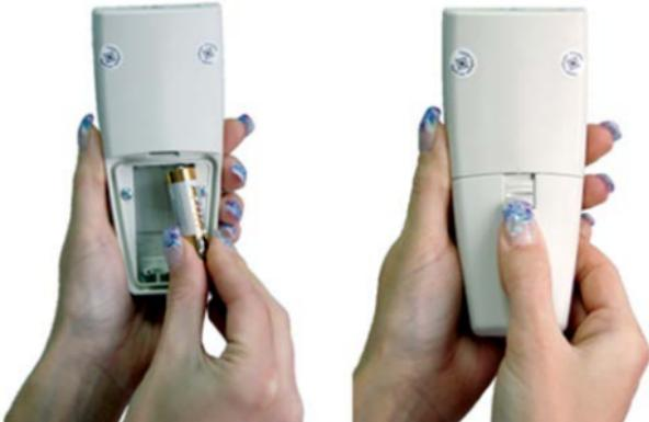
*Fig. 4. Changing the batteries*
